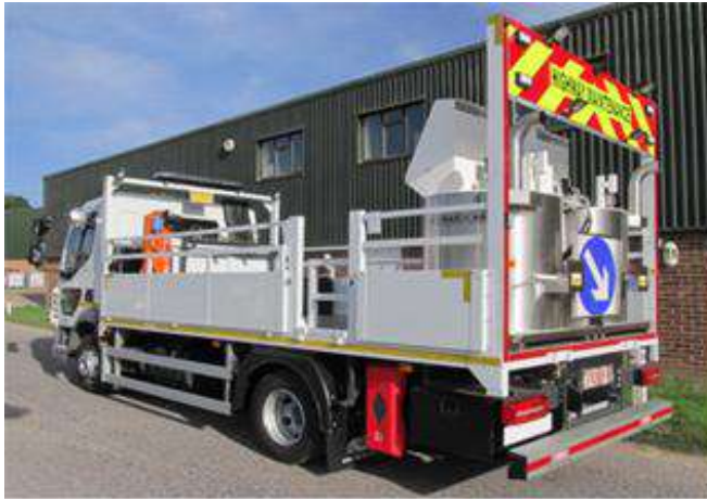
10 Tonne Screed Truck
