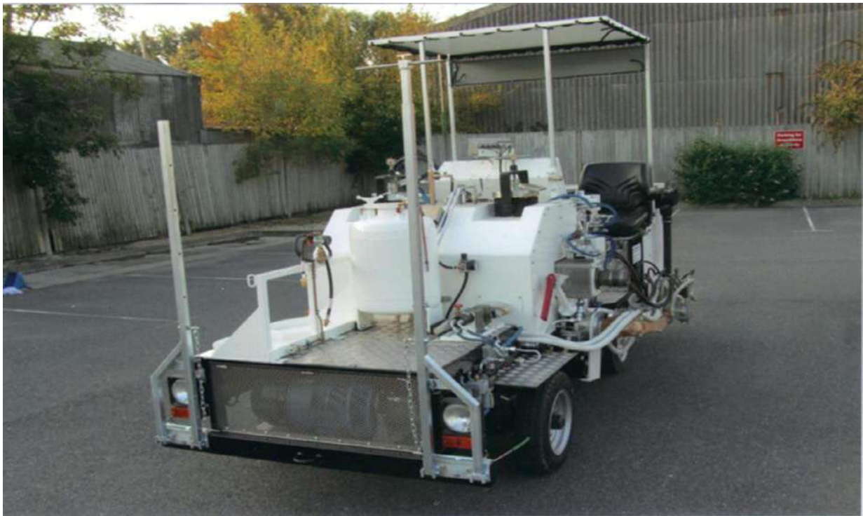
RM1100 Self Propelled Thermoplastic Spray/Extrusion Road Marking Machine
