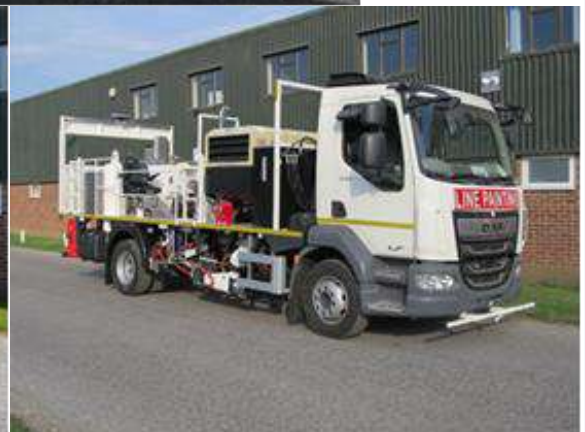
14 Tonne 5000 Spray and Extrusion Machine
