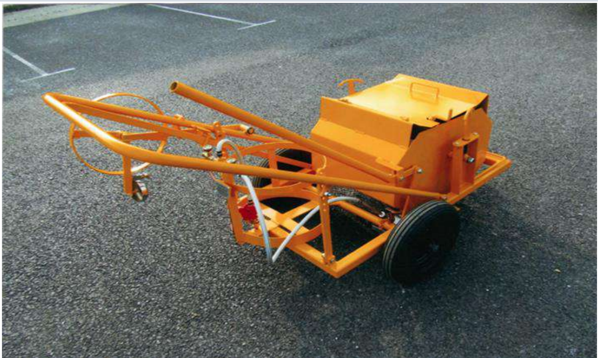
Pedestrian Operated Thermoplastic Screed Line Laying Machine
