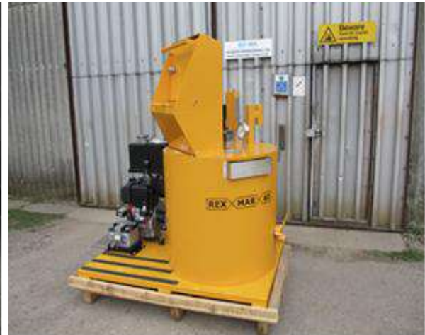
Single 1 x 40 Gallon Gas Fired Pre-Heater
